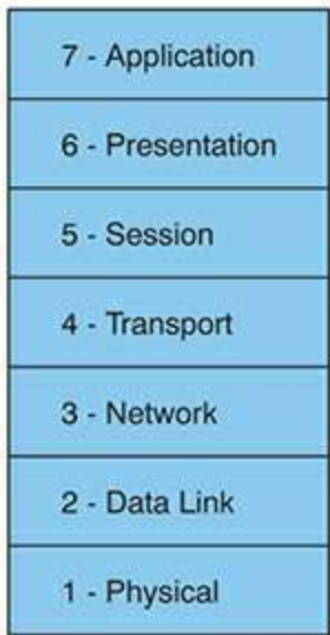
FIGURE 2.1 The OSI seven-layer model
