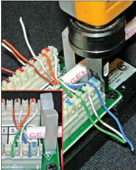
FIGURE 6.18 Punchdown tool inserting wires into an IDC
